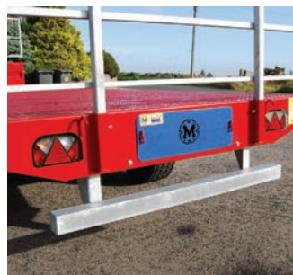
Recessed Lights, Rear Crash Barrier and Toolbox
