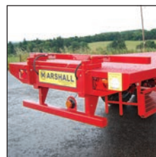
Rear Box Pusher & Hydraulic Walkway
